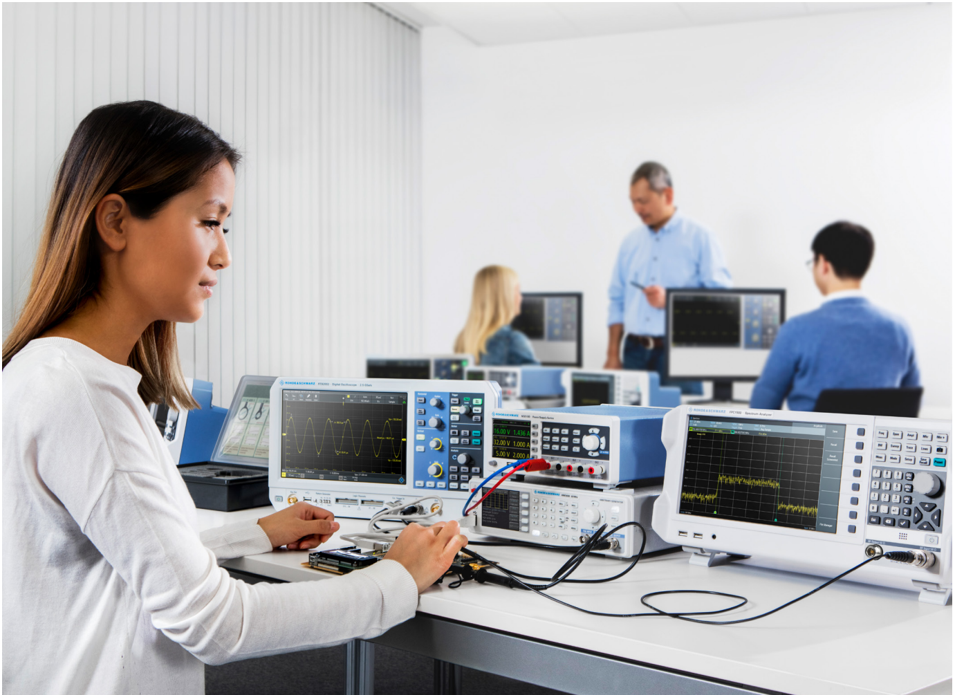
Typical university lab setup with the R&S®FPC1500, oscilloscope and power supply
